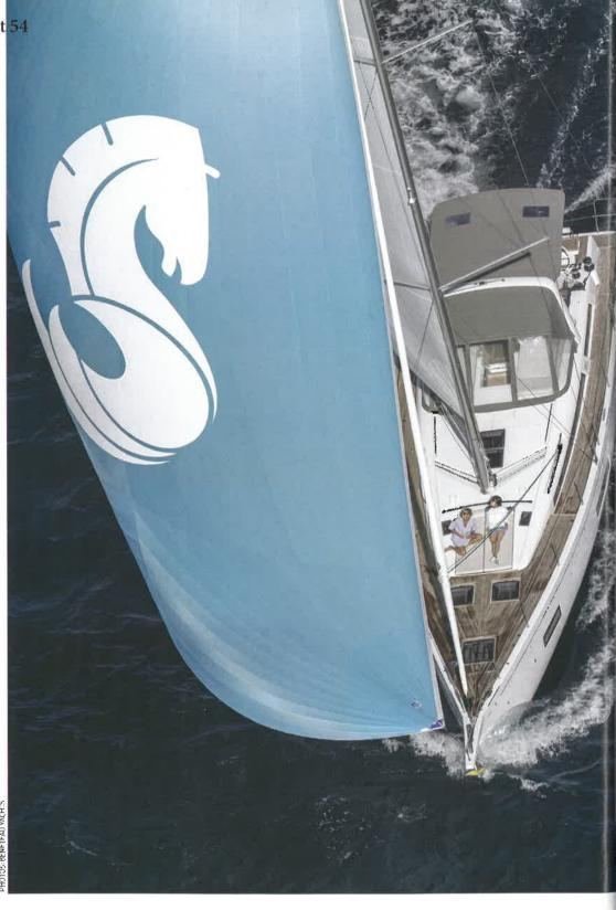
version available. The boat weighs in at 16,600kg, which makes her 1,100kg heavier than the First 53. The mast stepped rig is big but has been significantly reduced compared to her sportier sister. Perhaps the need to convert the hull of the 53 into a slightly more conservative 54 explains why the styling is not as aggressive as some of her direct competitors; there is a plumb bow rather than the dreadnought bow favoured by some manufacturers in this category.
