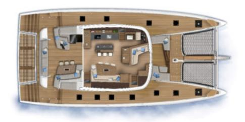
Access from the aft cockpit through a wide glazed sliding door (overall dimensions  $3.8 \times 1.95 \text{ m/12'6"} \times 6'5"$  - opening dimensions  $2.3 \times 1.95 \text{ m/7'7"} \times 6'5"$ )
