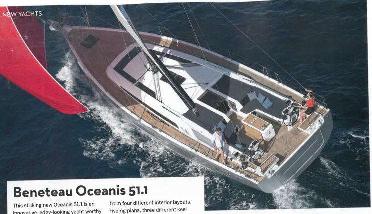
This striking new Oceanis 51.1 is an innovative, edgy-looking yacht worthy of a design award. The hull shape is full in the bows with a low spray rail chine in the forward sections.
