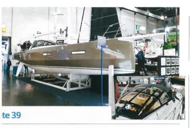
g a dash with its highly contemporary lines and radical panoramic roof, the new Bente 39 attracted plenty of attention at the show. It's based French Open Class concept and designed for long blue water cruising, the smaller Bente models which are coastal designs. The 39's hull has a ve double-bend bow and double chines, by Judel/Vrofijk & co. and the vings of modern ocean-going regatta yachts, such as the wide stern with 2 rudder and two steering positions.
